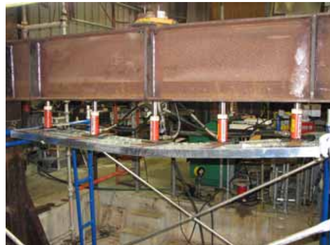
Uniform load application. Right photograph shows load at 5,325 lbs.
