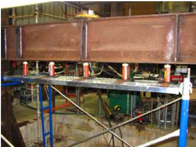
Uniform load application. Right photograph shows load at 5,325 lbs.
