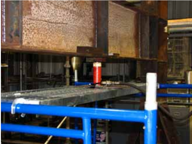
Point load application. Right photograph shows load at 1,375 lbs.
